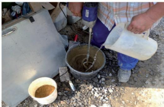
Preparation of a "bucket mixture" of RSS Flüssigboden® for the determination of the cubature
